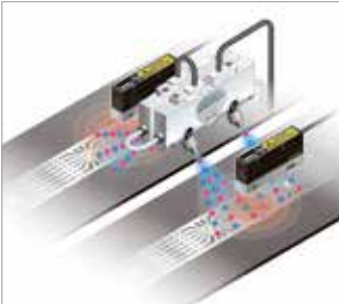
Measuring static electric charge in lead frames
