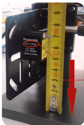
Example: HG-C1050-P Adjusted height 50mm
